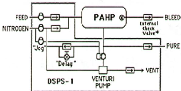
\*Required if unit does not have internal check valve in bleed line
